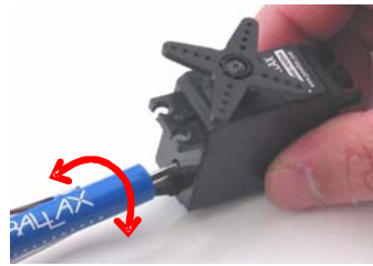
Figure 2-24 Center Adjusting a Servo
