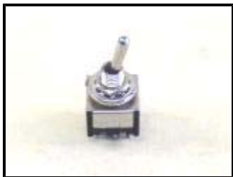
4) 1/4" Mini Power Switch (qty = 1) Note, may not have been included in early kits
