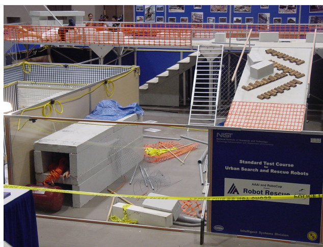
Figure 1: Part of the IJCAI Urban Search and Rescue Course. This course was constructed by NIST and was designed to simulate an urban disaster area. Teams earned points for locating and correctly identifying “victims” as well as notifying human operators of the victims’ locations.
