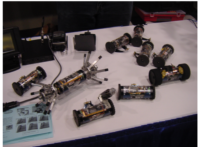
Figure 2: A collection of the Scout robots, including modified versions which have variable-sized wheels and low-light illumination abilities.
