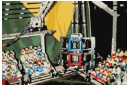
Figure4. The scoreboard and one of the small cameras. The camera runs up along the sideline, while projecting the images to a large monitor. ©H. H. Lund, 1998.
