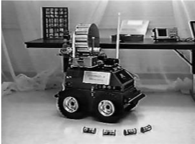
Figure 5: The distributed, reconfigurable robotic team. A four-wheeled ranger with scout launcher, radios, camera, and sonars is shown in the center of the figure. Four scouts are shown in the foreground.
