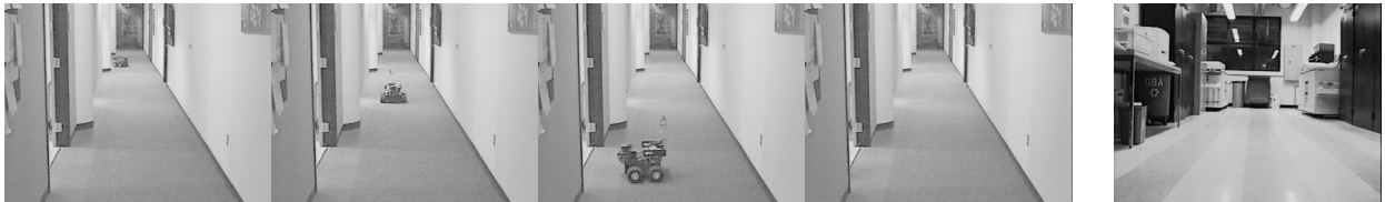
Figure 12: The Remote-Room-Inspection Mission (Trial-1): the robot entered the room since the red object was not present in the room.
