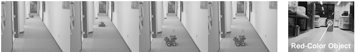
Figure 13: The Remote-Room-Inspection Mission (Trial-2): the robot stopped entering the room because the red object was detected.
