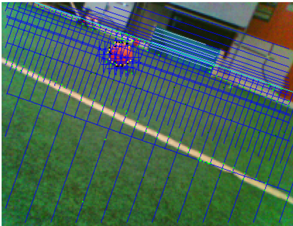
Figure 3.8: The complete scan line pattern with detected features displayed. Additional scan lines are constructed when few ball features are detected in the initial scan pattern. More features are most likely to be detected near existing features.
