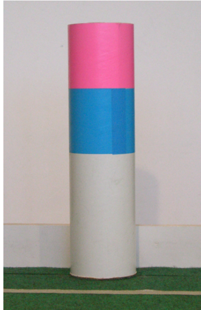
Figure 1.2: One of the four cylindrical beacons surrounding the field. Each has a unique combination of blue, yellow and pink coloured rings. These beacons can be used for self-localisation.
