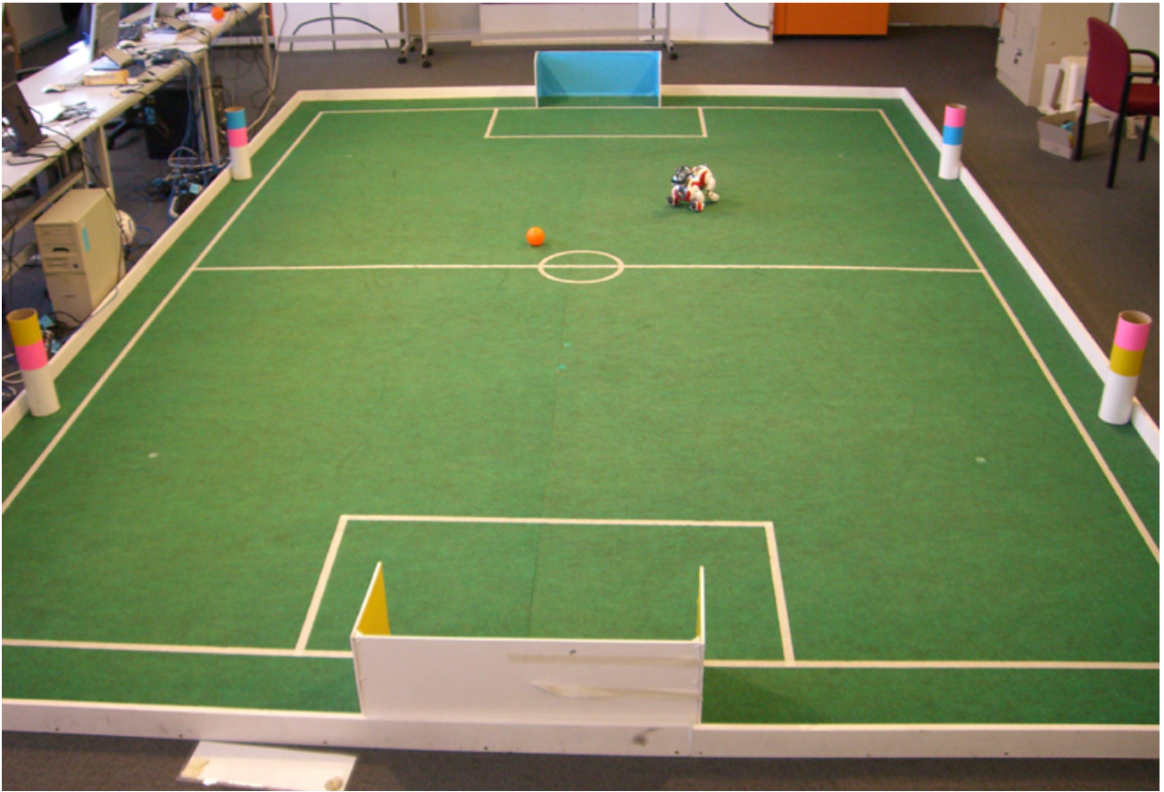
Figure 1.1: The RoboCup four-legged league field. Note the coloured goals and localisation beacons. The outer wall is optional.
