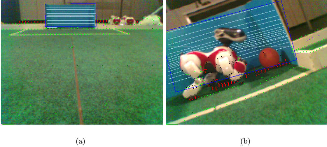
Figure 3.12: (a) A recognised goal. (b) The goal is often occluded by a robot, but grouping of features leads to correct recognition, even if the goal is divided in half. The two possible gaps for shooting are indicated by horizontal white lines. The recognised goal is assumed to be aligned with the horizon, so no attempt is made to detect the goal outline.
