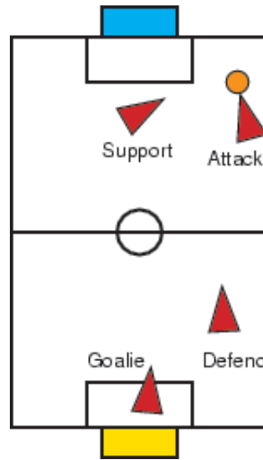
Fig. 4. Potential fields draw robots to their relevant field positions around the ball according to their roles.
