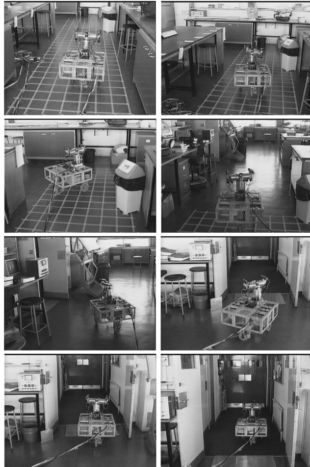
Fig. 12. The estimated trajectory and frames cut from a video as the robot navigated autonomously around two known landmarks and out of the laboratory door. The robot knew the locations of features 0 and 1 as prior knowledge, along with information on their status as obstacles.
