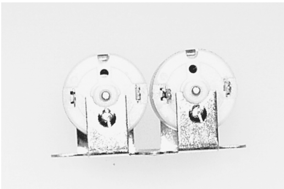
Figure 1-6 Motors installed in mounting bracket.
