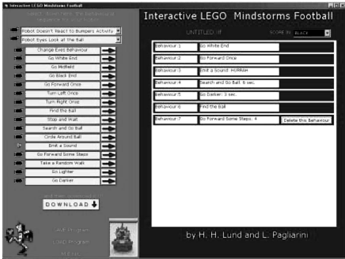
Fig. 11. The programming environment for LEGO MINDSTORMS RoboCup Junior. We used the behaviour-based approach, and developed primitives (the behaviours on the left), and allowed the children to make higher level strategies using these primitives. With this system, children from 7 to 14 years of age were able to develop their own robot footballers within 30–60 min. Copyright H.H. Lund and L. Pagliarini, 1999.
