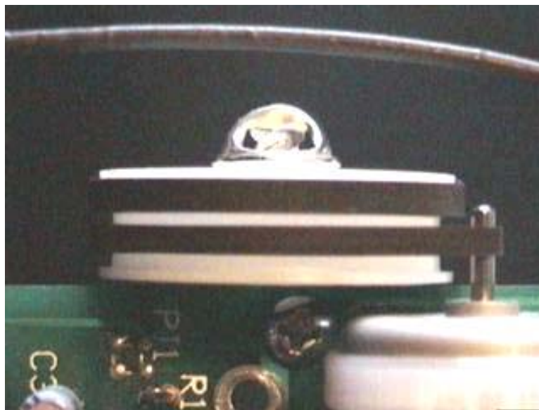
Figure 4. Correct belt alignment. Drive belt rides centered on top of ridge.
