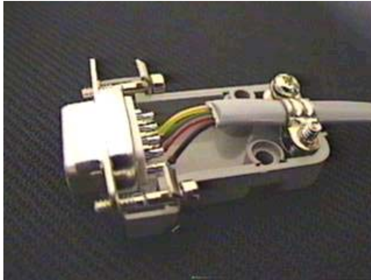
Figure 6. The wires should be loose with the strain relief in place in the hood
