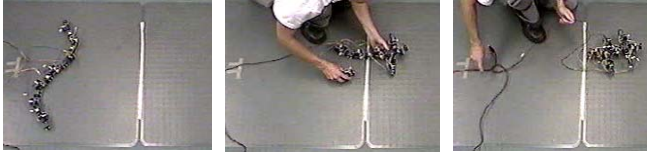
Figure 4. The robot first moves using a sidewinder gait (left). The robot is then manually reconfigured into a quadruped walker (middle). Finally the robot walks (right).
