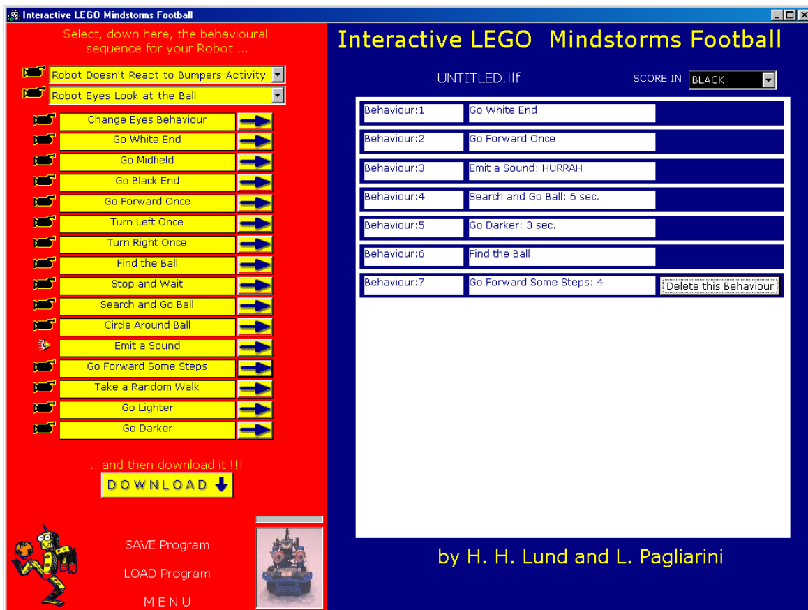
Figure 2. The programming environment for Interactive LEGO Football as used in RoboCup Junior. We used the behaviour-based approach, and developed primitives (the behaviours on the left), and allowed the children to make higher level strategies using these primitives. With this system, children from 7 to 14 years of age were able to develop their own robot footballers within 30-60 minutes. Copyright Lund and Pagliarini, 1999.
