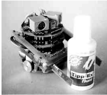
Fig. 4 Khepera robot with stereoscopic vision and gripper turrets.
