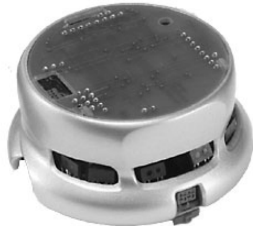
Figure 1. The Khepera II Robot.
